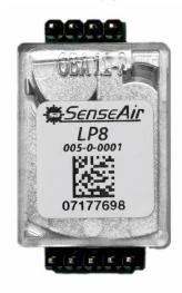
Senseair® LP8 is a miniature sensor module which targets battery-powered applications. It gives customer a full control on sensor integration into a host system, flexibility in changing of the CO<sub>2</sub> measurement, period and consequently power consumption. One measurement requires only 3.6mC of charge (or energy 11.9mJ at 3.3V battery supply). The sensor is supposed to be switched off between measurements to minimise power consumption.
